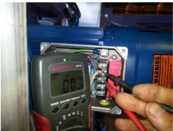
If there is 460v coming into the brake motor, the next check would be of the brake coil.
