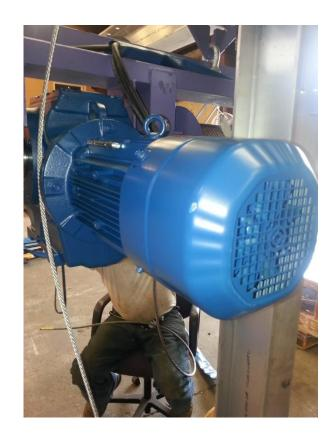
Loosen four screws holding motor cover and rotate Cover counterclockwise slightly to remove. 8mm
