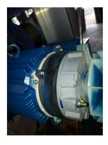
Screw into threaded port of brake coil housing.
