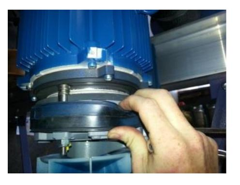
Roll back rubber seal to observe the 2 metal magnetic brake rings.
