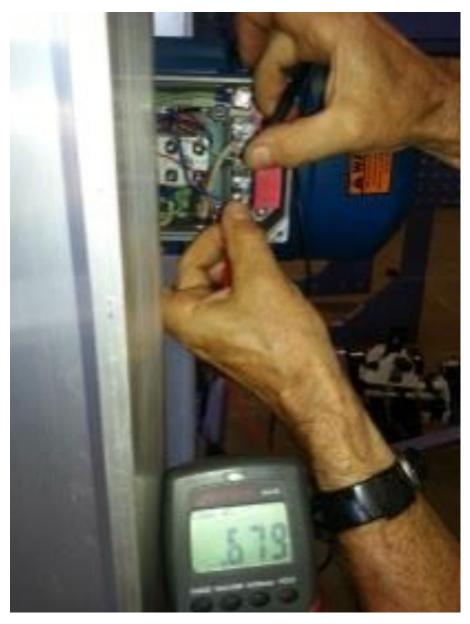
Next, check the small white and small blue wires using the mulitmeter.
