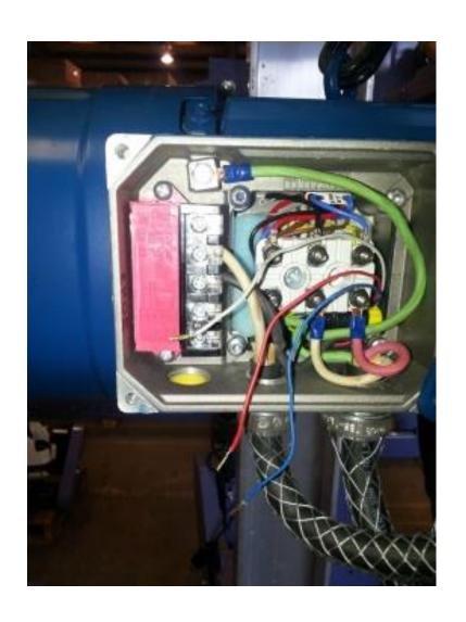
You first must loosen the 3 small wires from the rectifier. White from position 1, red from position 3 and blue from position 5.
