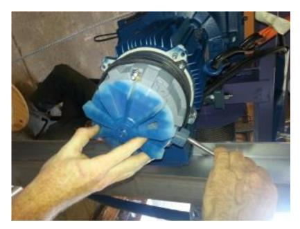
To insure brake motor is good, pull release handle and spin motor fan blade at same time. If fan spins, motor is ok, if does not spin, motor is bad and would need to be replaced.
