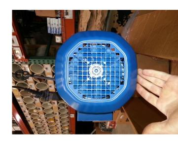
The simplest way to identify is by the motor fan guard. The "older" DT motor fan guard is round. The "newer" DRE motor fan guard is hexagonal.
